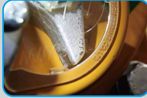
Heavily worn stopper
