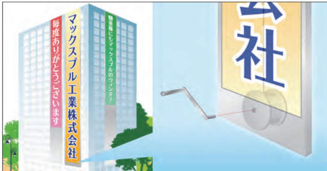
Small winch is used in the lifting equipment of vertical banner. It never spoils the landscape because it is not visible from the outside.
