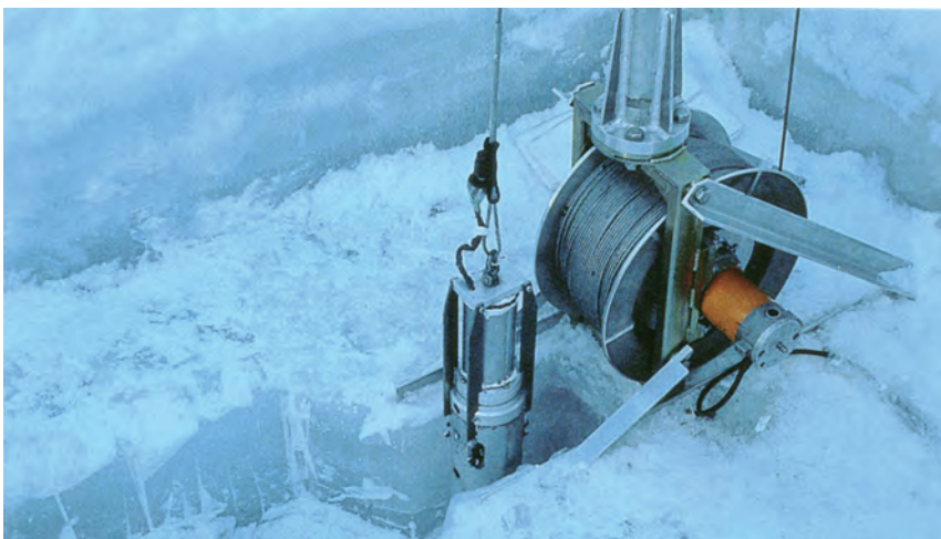
Antarctic Research "Electric winch MAW-1100 for deep ice coring system"
