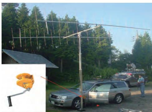
Disaster emergency radio relay antenna
