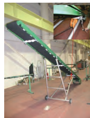
Belt conveyor angle adjustment
