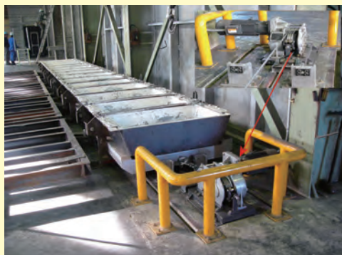
Pulling truck in both directions for carrying ingots in aluminum melting furnace
