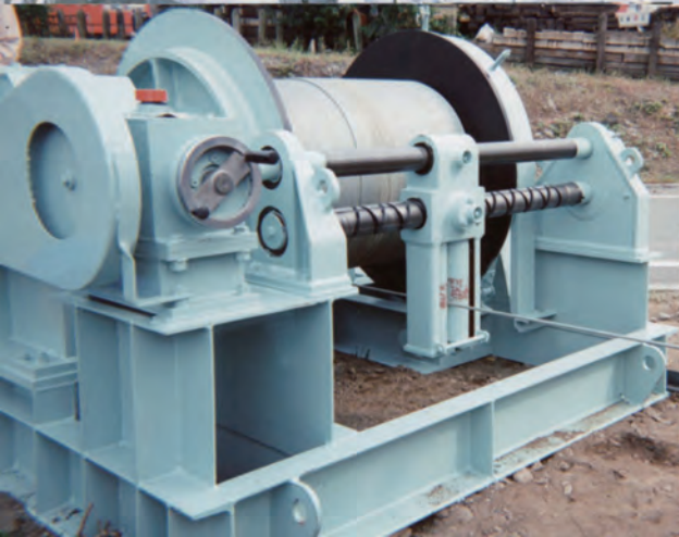
Antarctic Research "Electric winch MAW-1100 for deep ice coring system" for the 36th Japanese Antarctic Research Expedition
