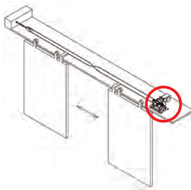
▲ Opening and Closing the Door in Airplane Hangar
